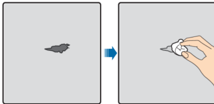
Figure 5: Treating the Damaged Coating with Anhydrous Ethanol
